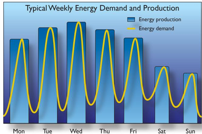
The ability of the hydroelectric project to generate electricity during periods of peak demand maximizes the value of the MFP.
